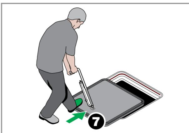
Align correctly with frame. Push cover into position using your foot.
